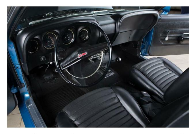
Base interiors featured the Mustang's standard gauge arrangement, which included alternator, fuel, temperature, and oil pressure gauges. Alternatively, when the option of a tachometer was selected, the Boss 302's alternator and oil pressure gauges were replaced with warning lights.
