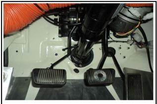
The Ford Falcon main outer tube will locate in the original lower firewall mount. An original Ford Australia coupler can then be used to join the collapsible inner shaft to the original steering box.
