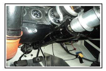
The original Ford USA steering column top and switches can then be mounted on the top of the Collapsible column to retain the original look and functions.
