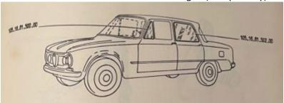
For 1970, updates included dual-circuit brakes, centre-mounted handbrake lever to replace under-dash "umbrella handle", larger external doorhandles, and top-hinged pedals (the latter in left hand drive models only; right hand drive continued with bottom-hinged pedals to the end of production (TI Super only).
